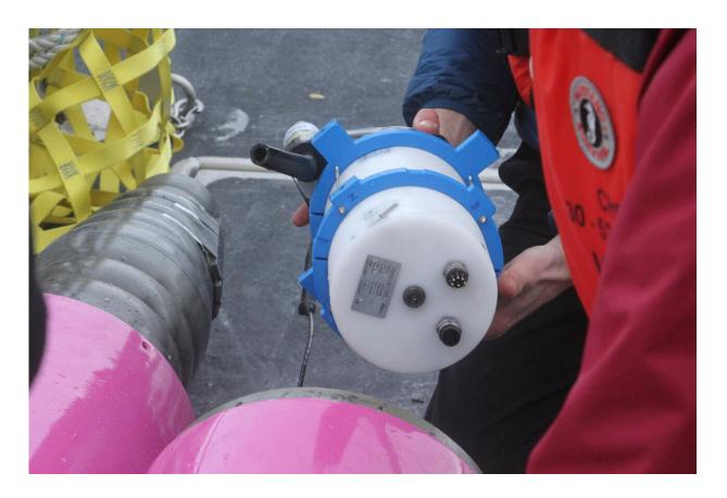
This May 4, 2022, photo shows a sensor after it was removed from an underwater glider on the University of Alaska Fairbanks research vessel Nanuq in the Gulf of Alaska. The glider was fitted with special sensors to study ocean acidification. Oceanographers from the University of Alaska Fairbanks tests have been conducting tests this spring with a drone that goes underwater, configured with a sensor specifically designed to measure carbon dioxide levels. Credit: AP Photo/Mark Thiessen
