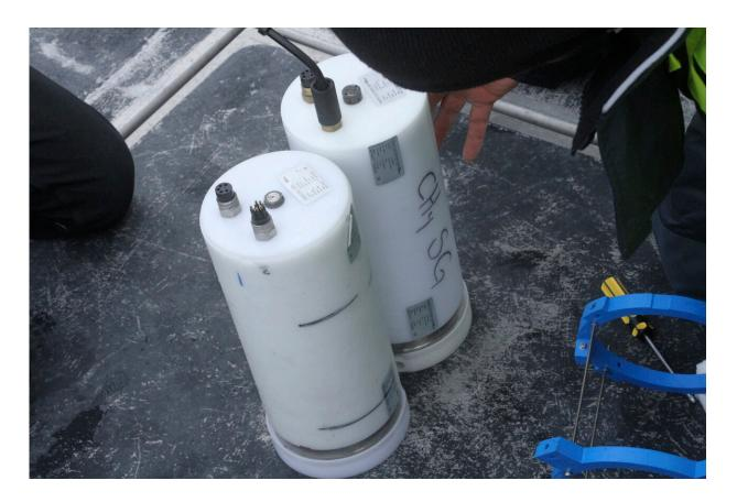
This May 4, 2022, photo shows sensors to measure carbon dioxide and methane, to be used separately on an underwater glider in the Gulf of Alaska. The glider was fitted with special sensors to collect an enormous amount of data to study ocean acidification. Credit: AP Photo/Mark Thiessen
