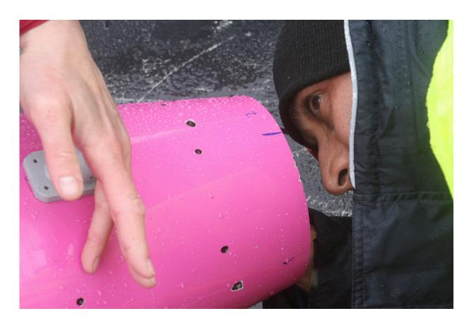
This May 4, 2022, photo shows engineer Ehsan Abdi looking from the other end as a sensor is placed inside an underwater glider on the University of Alaska Fairbanks research vessel Nanuq in the Gulf of Alaska. The glider was fitted with special sensors to study ocean acidification. Credit: AP Photo/Mark Thiessen
