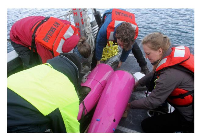
This May 4, 2022, photo shows an underwater glider being pulled apart on the University of Alaska Fairbanks research vessel Nanuq in the Gulf of Alaska to allow a sensor inside to be swapped out. The glider was fitted with special sensors to study ocean acidification. Credit: AP Photo/Mark Thiessen
