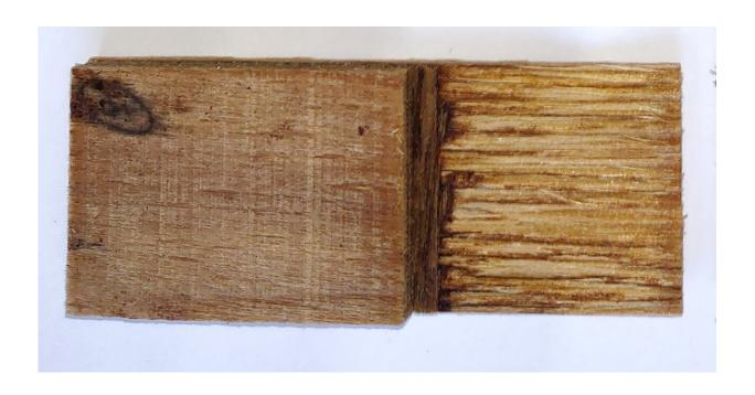
Citric acid and glucose produce a wood glue that creates strong, water-resistant three-layer plywood. Credit: Adapted from *ACS Applied Materials & Interfaces* 2022, DOI: 10.1021/acsami.2c02859
