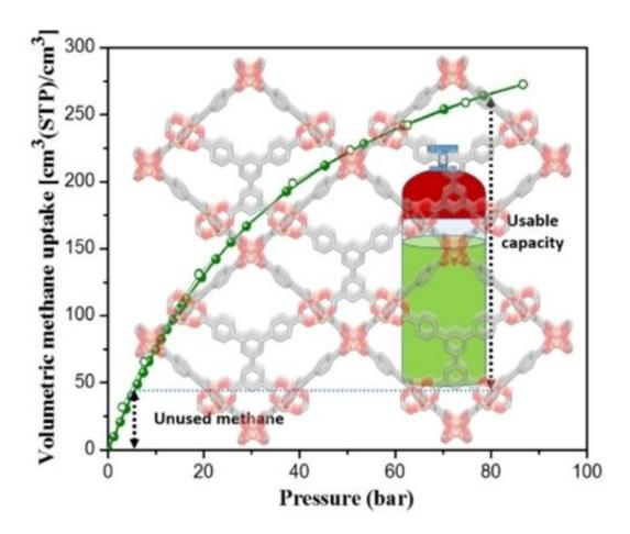
Promising MOFs were identified computationally and experimentally demonstrate remarkable methane uptake that outperforms known benchmarks both volumetrically and gravimetrically. Advanced set of interatomic potentials that explicitly accounts for the presence of coordinatively unsaturated sites (CUS) in MOFs were used to identify the high-capacity MOFs that were previously overlooked due to the limitation of the general interatomic potentials.
