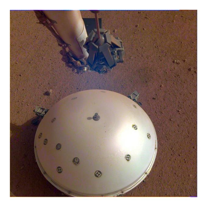
This image shows InSight's domed Wind and Thermal Shield, which covers its seismometer, called Seismic Experiment for Interior Structure, or SEIS. Credit: NASA/JPL-Caltech
