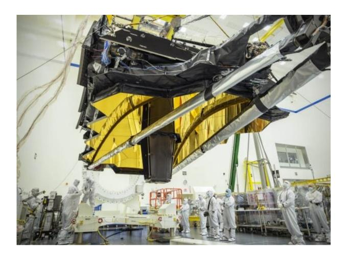
The sunshield of NASA's James Webb Space Telescope sits deployed inside a cleanroom at Northrop Grumman Aerospace Systems in Redondo Beach, California, in October 2017. Credits: Northrop Grumman
