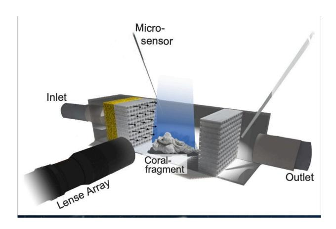
Watching corals breathe: A special camera records how oxygen sensitive particles flow past the coral surface. This allows the researchers to directly see the interaction between the flow field and oxygen concentration. Credit: Max Planck Society
