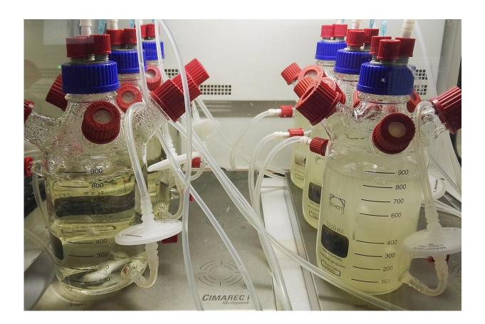
Loop reactor system: The five reactors with microbial communities were operated in the same way. The sixth reactor was connected to all five reactors. It synchronised the microbial communities and fed slow-growing bacteria back into the reactors. Credit: Zishu Liu / UFZ
