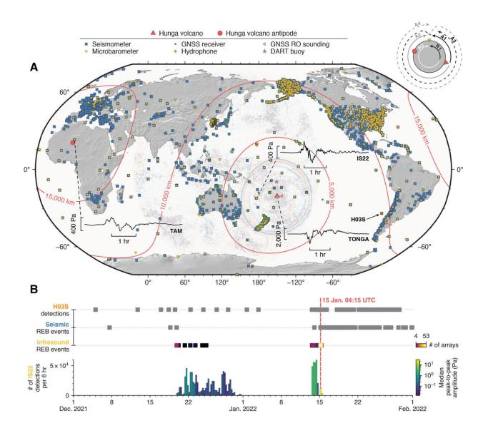
Global distribution of recording geophysical sensors used in this study and remotely-observed eruption chronology. (A) Sensor map. Background image is
