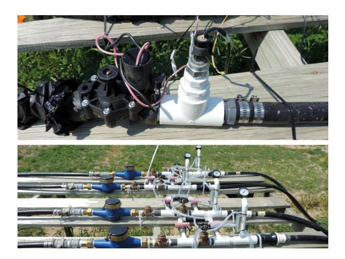
These photos show details of the set-up installed for the automation of the irrigation system in the experimental tomato field. Top is the electro-valve and pressure sensor; bottom is the fertigation manifold. For each treatment, the fertigation system included back-flow valve preventer, water meter to measure the water consumption, a Venturi fertilizer injector, a pressure gauge and a pressure regulator. Credit: Francesco Di Gioia/Penn State
