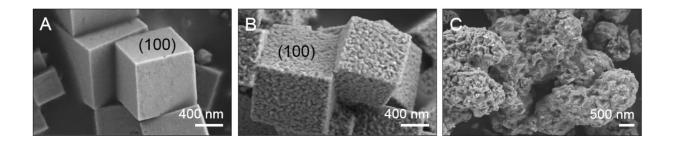
Scanning electron microscope images of the fresh Cu<sub>2</sub>O (A) and used catalyst for CC (B) and CLC (C) processes. Credit: IMCAS
