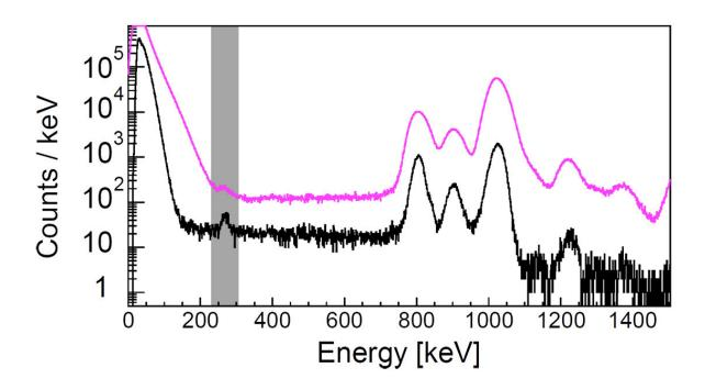
Proton detection data from the GADGET instrument. Readings from a single detector pad are shown in black and an aggregated signal from five pads is shown in pink. In both curves, several peaks are obvious above energies of about 800 keV, or kiloelectronvolts. What GADGET allowed researchers to detect was the important but tiny blip at the low energy of 260 keV (highlighted with a gray bar). Before these measurements, a proton peak this weak from this nuclear
