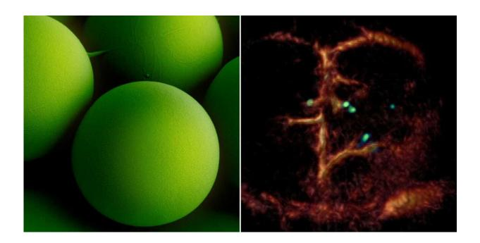
A breakthrough: Tiny circulating microrobots, which are as small as red blood cells (left picture), were visualised one-by-one in the blood vessels of mice with optoacoustic imaging (right picture). Credit: ETH Zurich / Max Planck Institute for Intelligent Systems
