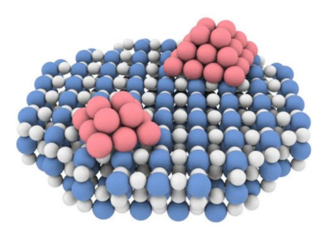
Schematic illustration for constructed Pd<sub>n</sub>/TiO<sub>2</sub>. Credit: Zhang Wenqing et al
