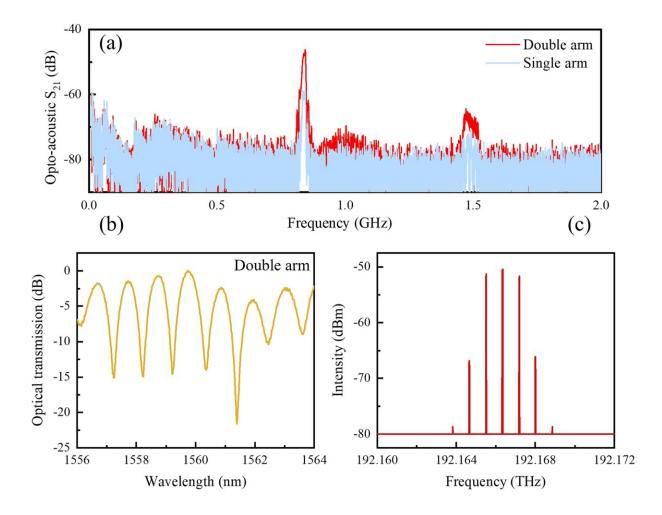
a S<sub>21</sub> spectra of the TFLN-ChG hybrid MZI-based AO modulators with single-arm and double-arm modulation configurations. b Normalized optical transmission spectrum of the AO modulator with the double arm configuration. c Measured optical sidebands in the push-pull AO modulator at an RF power of 15 dBm. Credit: by Lei Wan, Zhiqiang Yang, Wenfeng Zhou, Meixun Wen, Tianhua Feng, Siqing Zeng, Dong Liu, Huan Li, Jingshun Pan, Ning Zhu, Weiping Liu, and Zhaohui Li
