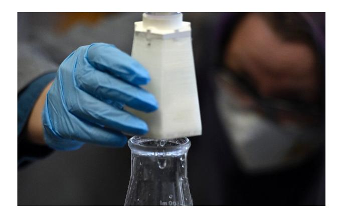
Using 3D printing and high-school level chemistry, a team of students and their teacher has produced a working prototype of an affordable and environmentally friendly filter to remove lead from water.
