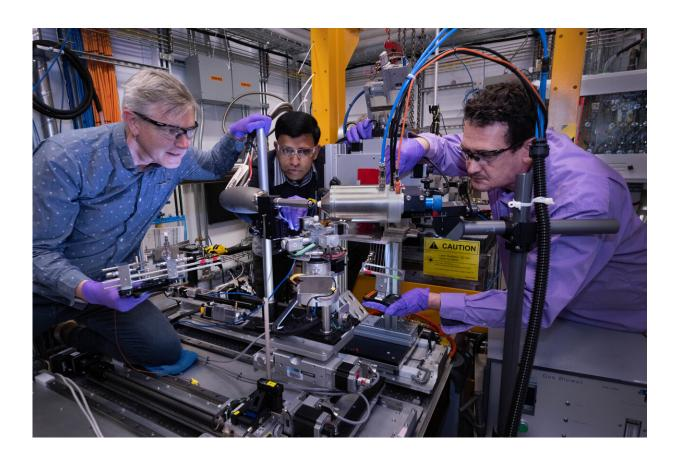
Brookhaven Lab members of the research team: Simon Billinge, Milinda Abeykoon, and Emil Bozin adjust instruments for data collection at the Pair Distribution Function beamline of the National Synchrotron Light Source II. In this setup, a stream of hot air heats samples with degree-by-degree precision as xrays collect data on how the material changes. Credit: Brookhaven National Laboratory
