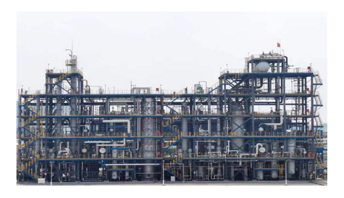
The industrial facility of 50 kt/year propanal/n-propanol by heterogeneous ethylene hydroformylation. Credit: LI Cunyao
