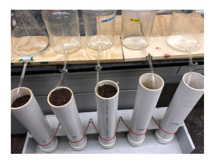
The study looked at artificial rainwater soaking experiments with different materials in the bioretention cells to test for a better way to build bioretention cells. The tests differed in their composition of sand, soil, zeolite, and peat moss. One finding was that zeolite helped water soak in faster, and it retained more nitrogen than typical materials. Credit: Caitlin Sweeney
