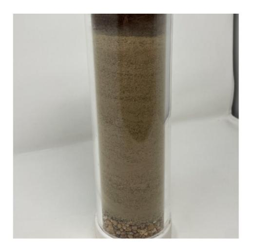
A cross-section of a bioretention cell with aquarium gravel on the bottom, a bioretention mix and peat moss on top. These ingredients were used to measure how effective rain gardens can absorb water runoff. Credit: Thorsten Knappenberger
