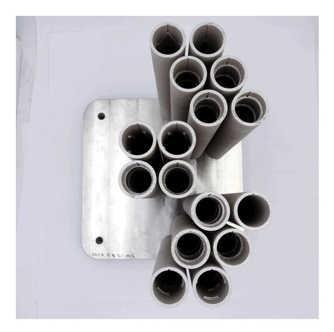
3D-printed tubes produced at MDF, showing different flow disturbance
