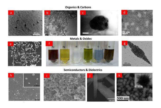
Types of nonlinear optical nanoparticles fabricated by laser ablation. Credit: Compuscript Ltd
