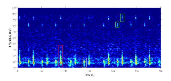
Spectrogram of example vocalizations of the fin whale. The 20 Hz pulse (red box), the back-beat pulse (white box) and the higher-frequency components accompanying both the back-beat and 20 Hz pulses (green boxes). Image was taken from Cape Leeuwin, (06-Aug-2011, 19:00). Spectrograms were calculated in 256-point Hann windows with 0.49 frequency resolution; sampling frequency 250 Hz. Credit: *Frontiers in Marine Science* (2022). DOI: 10.3389/fmars,2022.864153
