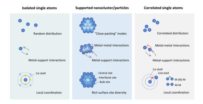
C-SACs with metal-metal interactions. Comparison of C-SACs with the conventional isolated SACs and supported metallic cluster/nanoparticle catalysts from the perspective of spatial distribution, intersite interactions, and local coordination. Credit: *Science Advances* (2022). DOI: 10.1126/sciadv.abo0762
