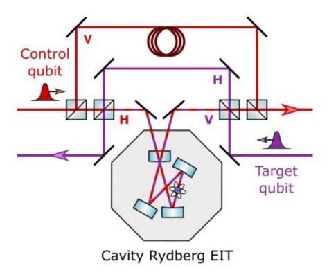
Experimental setup. Depending on the initial state of the qubits, the photons travel along different paths, some of which are reflected by the resonator. In this path, the photons experience an interaction, which is mediated by Rydberg states. Credit: Max Planck Society
