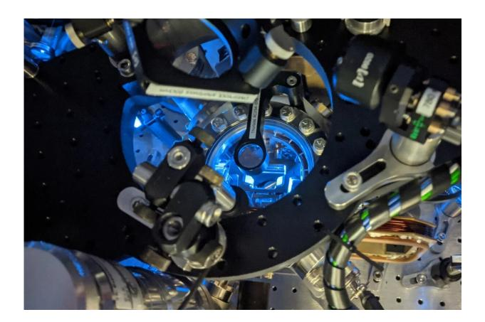
Photo of the vacuum chamber. Through the window into the vacuum chamber in the centre of the picture, one can see the holder for the mirrors of the resonator. Between the mirrors, ultracold atoms generate the interaction between the photons. Credit: Max Planck Society
