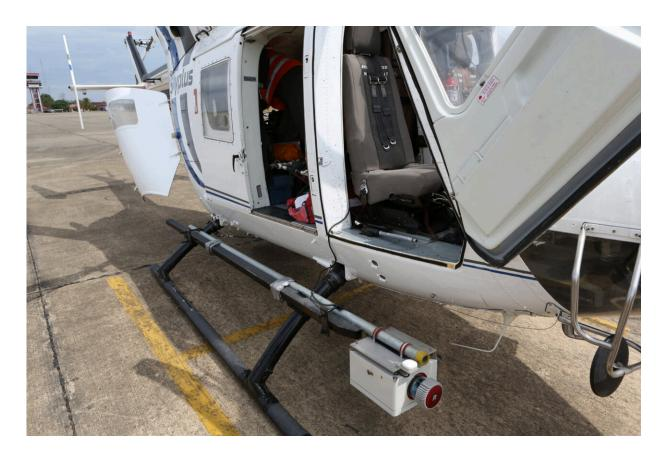
The Lidar scanner, attached to the helicopter. Credit: Heiko Prümers / DAI
