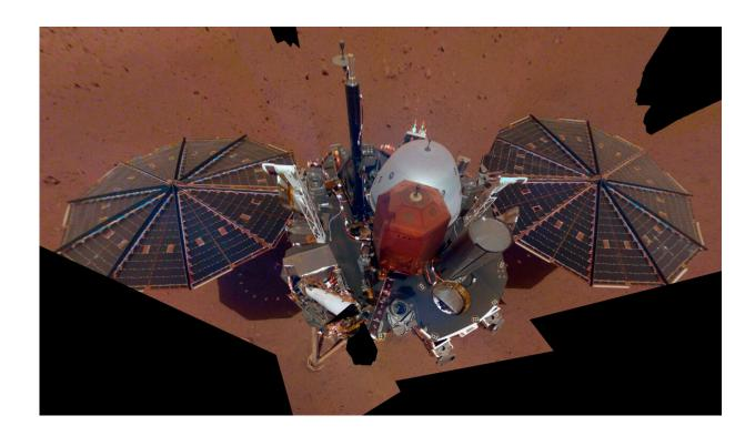
This Dec. 6, 2018 image made available by NASA shows the InSight lander. The scene was assembled from 11 photos taken using its robotic arm. The spacecraft is losing power because of all the dust that's accumulated on its solar panels. NASA said Tuesday, May 17, 2022, it will keep using the spacecraft's seismometer to detect marsquakes until its power peters out. Officials expect operations to cease in July, almost four years after InSight's arrival at Mars. Credit: NASA via AP, File
