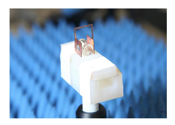
Copper "headphones" boost the sensitivity of NIST's atomic radio receiver, which is composed of a gas of cesium atoms prepared in a special state inside the glass container. When an antenna located above the setup sends down a radio signal, the headphones boost the strength of the received signal a hundredfold. Credit: NIST
