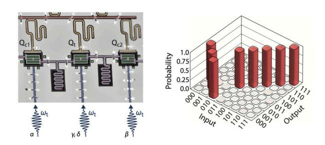
Experimental schematic of the high-fidelity iToffoli gate at the Advanced Quantum Testbed. Credit: Yosep Kim/Berkeley Lab
