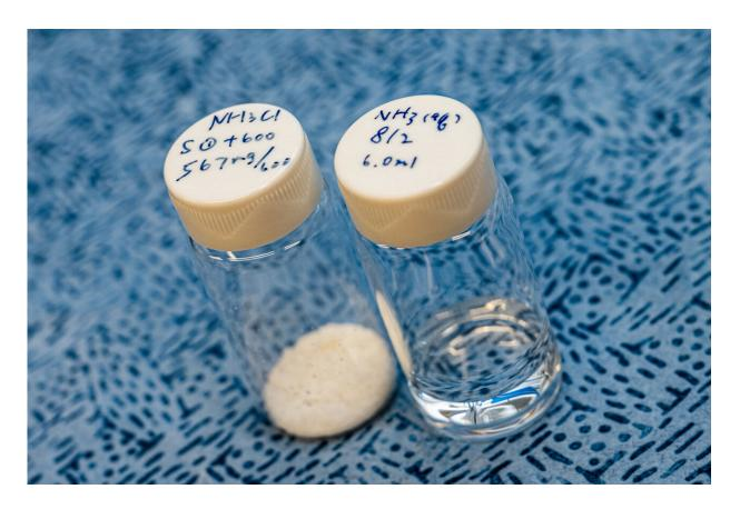
Ammonium chloride, at left, and liquid ammonia are the products of a catalyst developed by engineers at Rice University to convert wastewater into useful chemicals. Credit: Jeff Fitlow/Rice University
