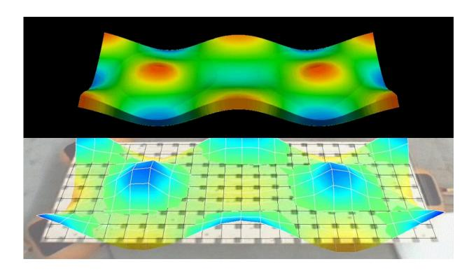
Intelligent noise insulation: Calculations of the vibration of wood panels with "black holes." Credit: Empa
