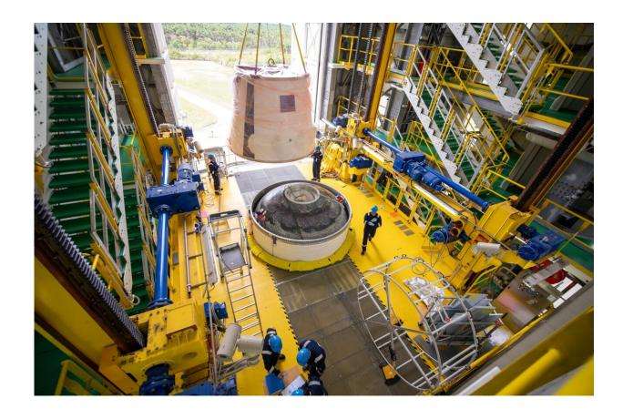
The Vega-C Interstage 1/2 has now been transferred to and integrated at the Vega Launch Zone (Zone de Lancement Vega) ZLV at Europe's Spaceport in Kourou, French Guiana on 22 April 2022. Credit: ESA/CNES/Arianespace/Optique video du CSG/P Baudon
