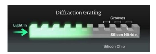
The NIST team directed light into an ultrathin layer of silicon nitride etched with grooves to create a diffraction grating. If the separation between the grooves and the wavelength of light is carefully chosen, the intensity of light declines much more slowly, linearly rather than exponentially. Credit: S. Kelley/NIST
