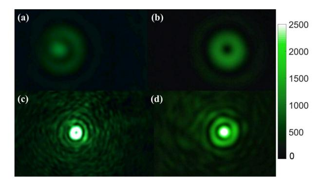
Fig. 3 The tightly focused light fields of (a) radially polarized beam; (b) azimuthally polarized beams; (c) radially polarized beam with 1-order vortex phase; (d) azimuthally polarized beams with 1-order vortex phase. Credit: Compuscript Ltd
