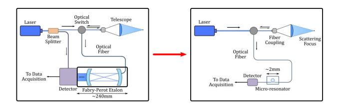
Left: Image of the Fabry-Perot LiDAR. Right: A representation of the whispering gallery mode (WGM) optical microresonator and how it would work. Credit: Elie R. Salameh, Southern Methodist University (SMU)
