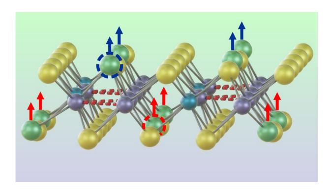
A side-view rendering of molybdenum disulfide, a technologically appealing material that consists of two sulfur atoms (yellow and green) for every one molybdenum (purple and blue). Nebraska researchers found that the upward shift of the green sulfur atoms contributes to the emergence of ferroelectricity, a prized but rare property that can help encode digital data using substantially less power. Credit: Alexey Lipatov / *npj 2D Materials and Applications*
