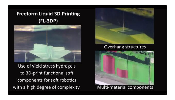
Use of yield stress hydrogels to 3D-print functional soft components for soft robotics with a high degree of complexity. Credit: SUTD
