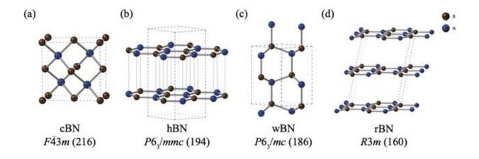
The structures and space groups of (a) zinc-blende boron nitride (cBN), (b) hexagonal boron nitride (hBN), (c) wurtzite boron nitride (wBN), and (d) rhombohedral boron nitride (rBN). Boron and nitrogen atoms are depicted in brown and blue, respectively. Credit: Kousuke Nakano from JAIST.
