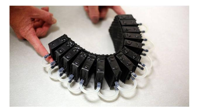
The soft-robotic assistive actuator prototypes work by using gas pressure to expand the internal chambers, causing them to bend. Credit: Texas A&M Engineering
