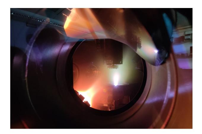
Pulsed laser deposition: An intense laser pulse hits a target containing the material, tranforming it into a plasma which is then deposited as a thin film onto a substrate. Credit: R. Gottesman/HZB
