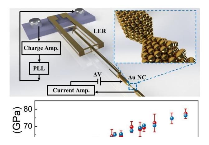
(Top) The nanomechanics measurement set-up. (Bottom) Young's modulus of Au nanocontacts plotted as a function of cross-sectional area. Red circles represent experimental values and blue circles indicate results from firstprinciples calculations. (Inset) a typical TEM image of an Au nanocontact. Credit: Yoshifumi Oshima from JAIST.
