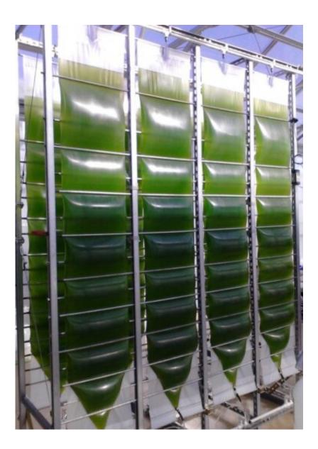
The air accordion photobioreactor that Joel Cuello and his biosystems engineering team designed. This photobioreactor will be further optimized to
