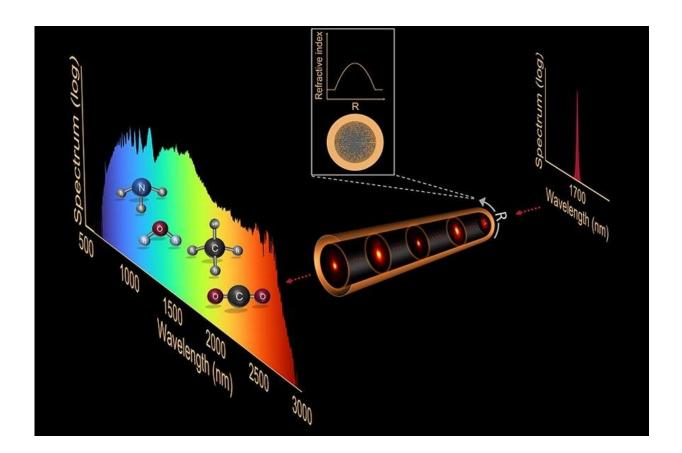
Utilizing two glasses with a different refractive index and stacked with a specific arrangement has allowed researchers to develop for the first time a multimodal fiber with a parabolic refractive index with transmission up to the mid-infrared and high nonlinearity. The spectrum of short pulses of light injected into the fiber massively broadens to span from the visible to mid-infrared. Significantly, unlike in conventional multimode fibers, the light beam remains smooth as the
