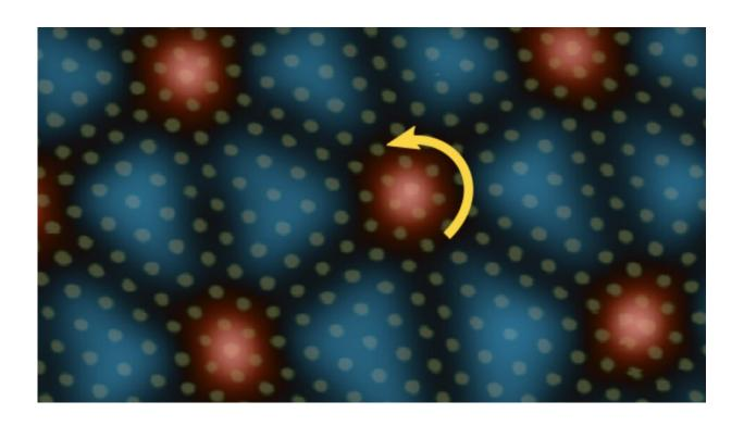
In the three layers of graphene depicted here, local twist angle can range from around 1.5 degrees (blue)—close to the "magic angle" for this device—to around 1.9 degrees (red). The arrow shows a twist angle vortex, or twiston. These areas of disorder help make the overall device more orderly. Credit: Simon Turkel
