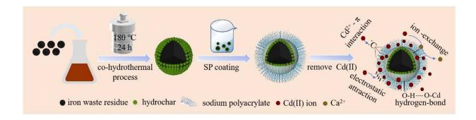
Schematic diagram of the fabrication process and the adsorption mechanisms of OWIR@TWL@SP. Credit: WU Qingchuan
