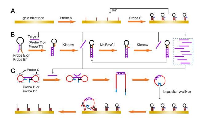
Electrochemical sensing strategy based on looped bipedal DNA walking. Credit: Miao et al.
