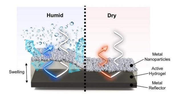
Schematic diagram and the principle behind ultrafast full-color colorimetric humidity sensor. Credit: POSTECH
