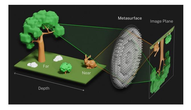
Illustration of how the metalens modeled on the compound lens of a trilobite simultaneously focuses object both near (rabbit) and far (tree). Credit: S. Kelley/NIST
