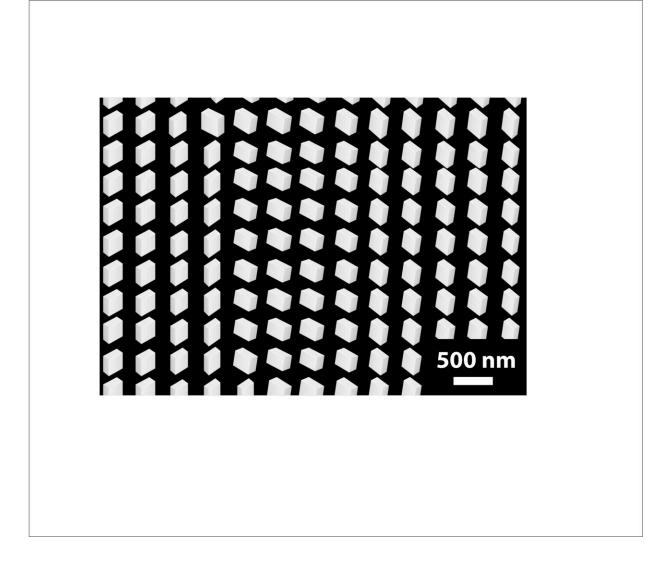
Scanning electron microscope image of the titanium oxide nanopillars that make up the metalens. The scale is 500 nanometers (nm). Credit: NIST
