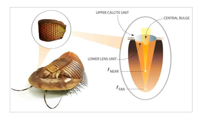
Inspired by the compound eyes of a species of trilobite, researchers at NIST developed a metalens that can simultaneously image objects both near and far. This illustration shows the structure of the lens of an extinct trilobite. Credit: NIST
