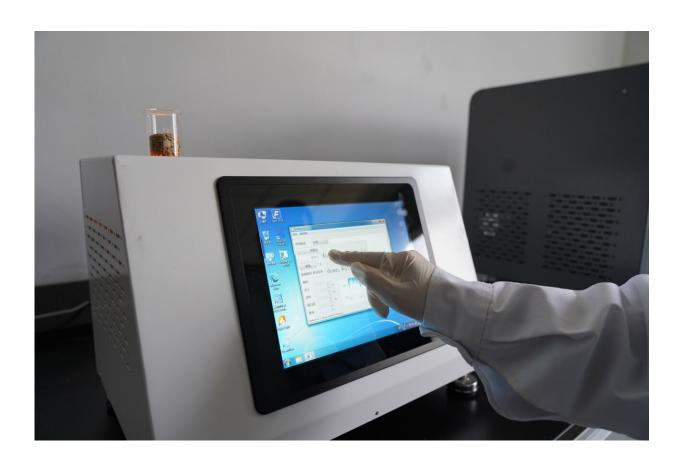
Portable Cereal Quality Rapid Detector basing on Near-infrared spectroscopy realized rapid and accurate detection of cereal quality. Credit: Zhao Weiwei
