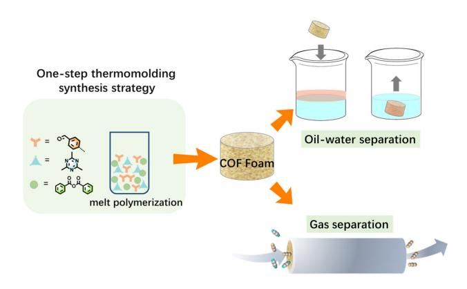
Construct covalent organic frameworks foam separators by melt polymerization. Credit: Science China Press
