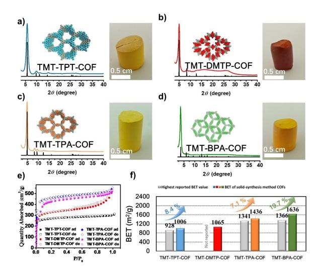
(a-d) Characterization of COF foams by PXRD. (e) Nitrogen adsorption curves of COF foams at 77 K. (f) Comparison of BET surface areas for the four COFs (gray columns for reported COFs; colored columns for COF foams in this study). Credit: Science China Press
