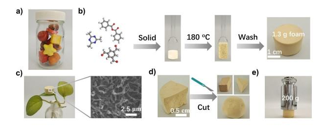
(a) COF foams with different shapes. (b) Scheme of the one-step synthetic procedure for gram-scale preparation of NKCOF-12. (c) Left: A photograph of NKCOF-12 foam standing on a leaf. Right: SEM image of NKCOF-12 foam. (d) The image of different shapes processed from NKCOF-12 foam. (e) A photograph of NKCOF-12 foam under compression. Credit: Science China Press
