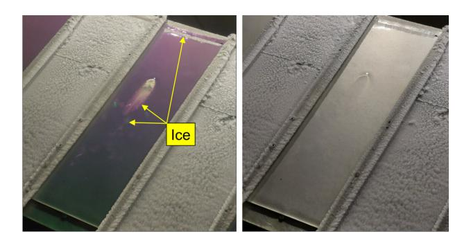
Ice forming on an aluminum plate in a weather chamber as seen with the approach proposed in the study (left) and with the naked eye (right). Credit: Viktor Grishaev et al./Cold Regions Science and Technology
