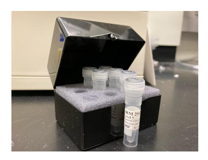
SRM 2917, Plasmid DNA for EPA-Developed Fecal Indicators, is a standardized reference material that contains 13 genetic markers, known DNA sequences, that can be used to identify a pollution source or estimate the concentration of fecal pollution in a sample. Credit: J. Kralj/NIST
